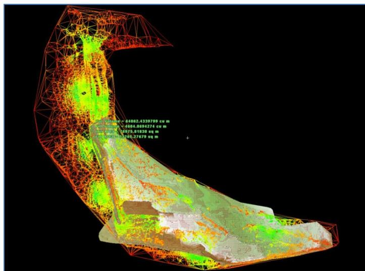
**Fig. 7 A comparison of the two surface models to derive the common area and the elevation differences between April and May**
