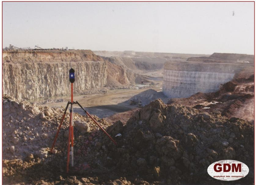
Fig.1 Laser Scanning Target at an Aggregate Mine
